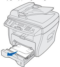
If there is any resistance when you pull the paper, or the paper is not seen in this area, continue with the instructions for clearing a jam in the fuser and toner cartridge areas on page 77.
